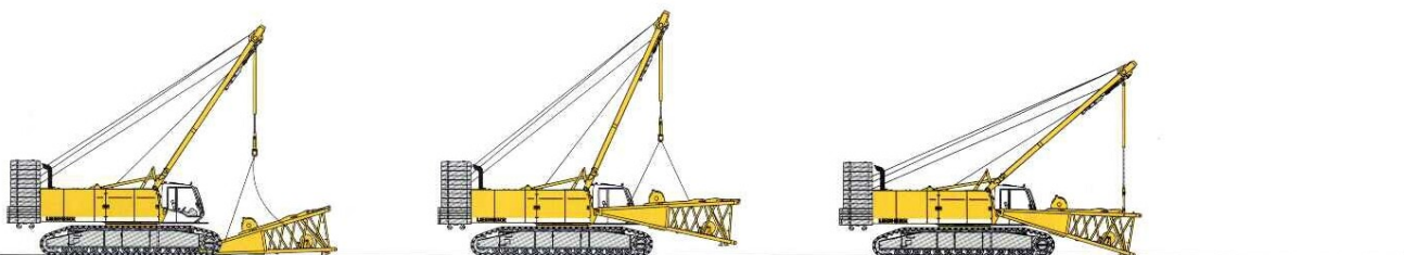
Unloading and assembly of boom foot
