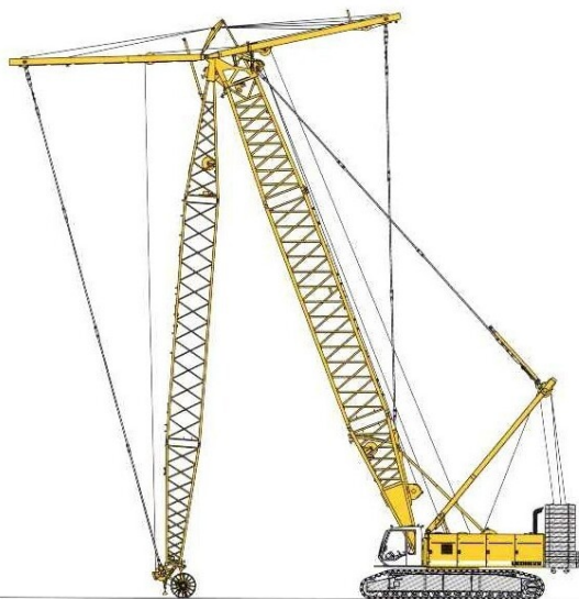
Erecting of main boom and luffing jib
