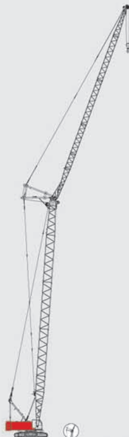
主臂 Boom 塔臂 Luffing jib 25.8m-43.8m 21m-39m
